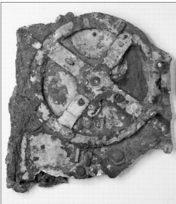
Fig. 1 Antikythera Mechanism, fragment A (the largest fragment), front face. The spoked wheel, one turn of which represents one year; measures about 130 mm. in diameter.
