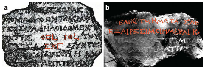
Figure 1 | The 'instruction manual'. Previously identified inscriptions 1,6 reveal remnants of an instruction manual, describing the Mechanism's cycles, dials and functions, as seen in two examples from the Mechanism's back dial. a , Polynomial texture mapping of fragment 19 shows fine surface detail, with text about 2 mm high. Highlighted in red are “76 years, 19 years” for the Callippic and Metonic cycles (Supplementary Box 1), and “223”, for the Saros cycle (Supplementary Box 2). b , X-ray CT of fragment E reveals text about 2 mm high. Highlighted are “on the spiral subdivisions 235”, confirming the Metonic dial (Supplementary Box 1); and “excluded days 2...”, the final “K” presumably standing for the number 20—part of the 22 excluded days round each of the five turns of the Metonic calendar—though “B” that would complete “KB” (22) remains speculative.
