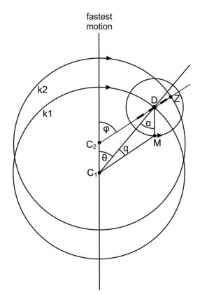
FIG. 2. Pin-and-slot mechanism for the lunar inequality in the Antikythera mechanism, compared with the epicycle-plus-concentric theory in the standard astronomy of Hipparchos or Ptolemy.
