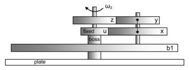
FIG. 7B. A second way to get wheel z rotating at the mean sidereal frequency of a superior planet, using a stationary boss.
