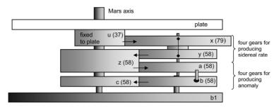
FIG. 10. Complete solution for Mars, embodying the correct sidereal period and the correct anomalistic period. Seven gears in all are used.
