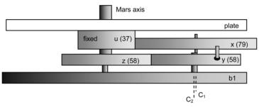
FIG. 12A. Four-gear solution equivalent to Fig. 10. Stationary gear mounted to a plate nearer the front of mechanism.
