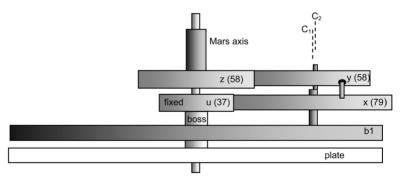
FIG. 12B. Alternative four-gear solution, with stationary gear mounted on a boss fixed to the plate behind b1.
