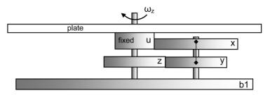
FIG. 7A. One way to get wheel z rotating at the mean sidereal frequency of a superior planet. The example is for Mars, with u, x, y, z = 37, 79, 58 and 58 teeth.
