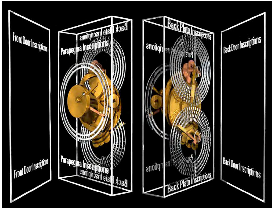
Supplementary Figure 2 | Schematic showing the overall architecture of the Mechanism in a 2006 model 6 . The present model revises the Back Dials: the function of the upper subsidiary dial and the geometry of the main lower dial.
